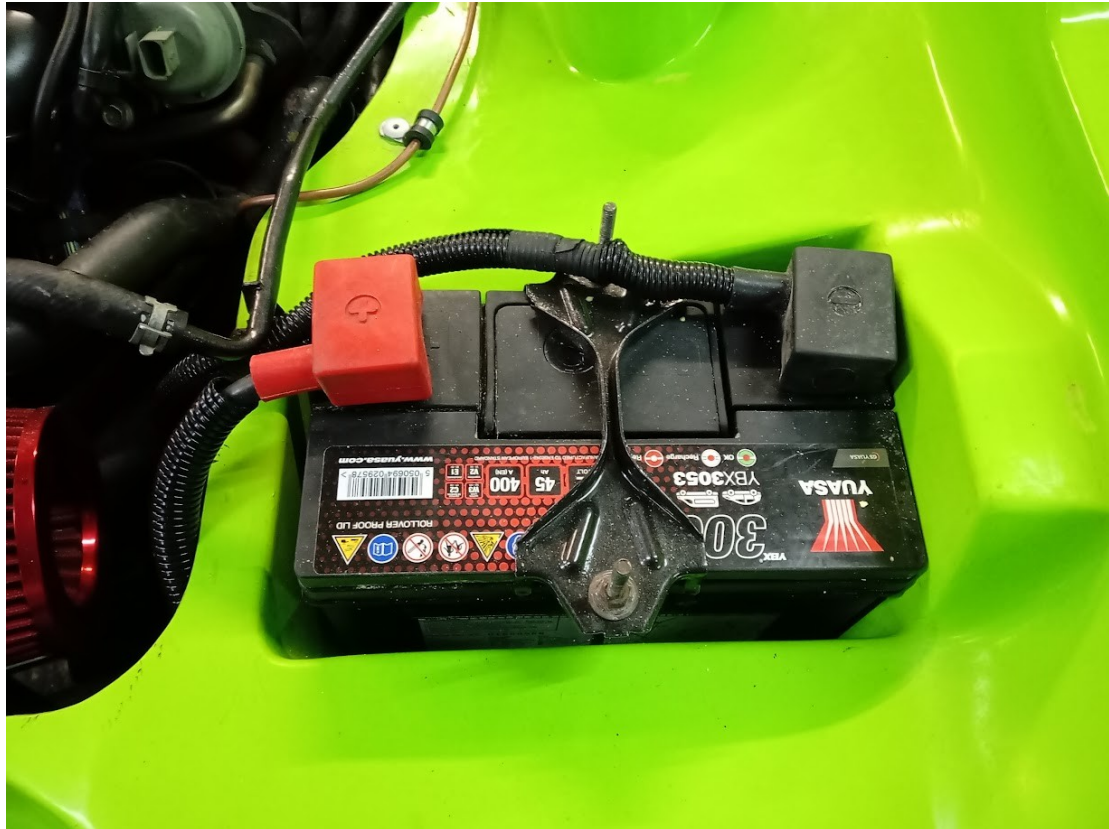
Fit standard Mazda battery and attach with Mazda battery clamp. Fit both terminal covers
