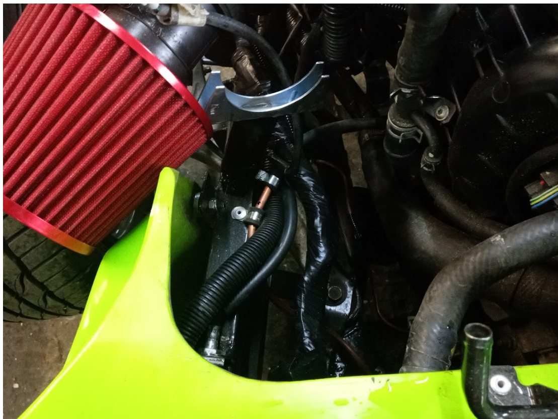
Bolt air filter to bracket welded onto top of chassis. Note position of fuel pipe bundy and riveted P clip
