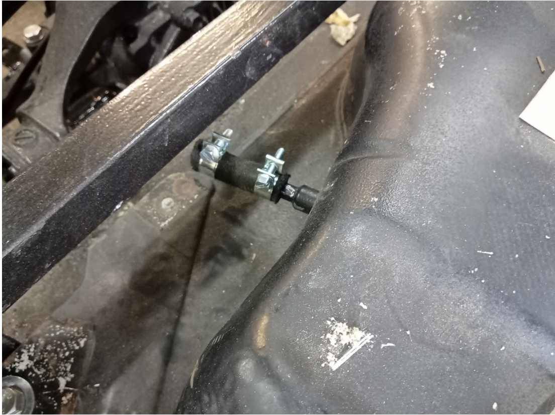
Blank off unused tank vent with hose/ blanking plug and clips ABS
