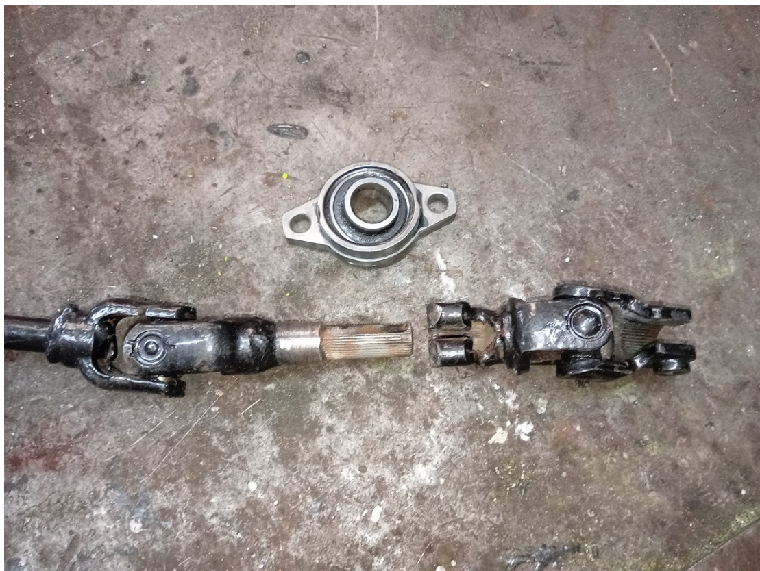
Factory modified steering column, self aligning bearing and rack U/J.
