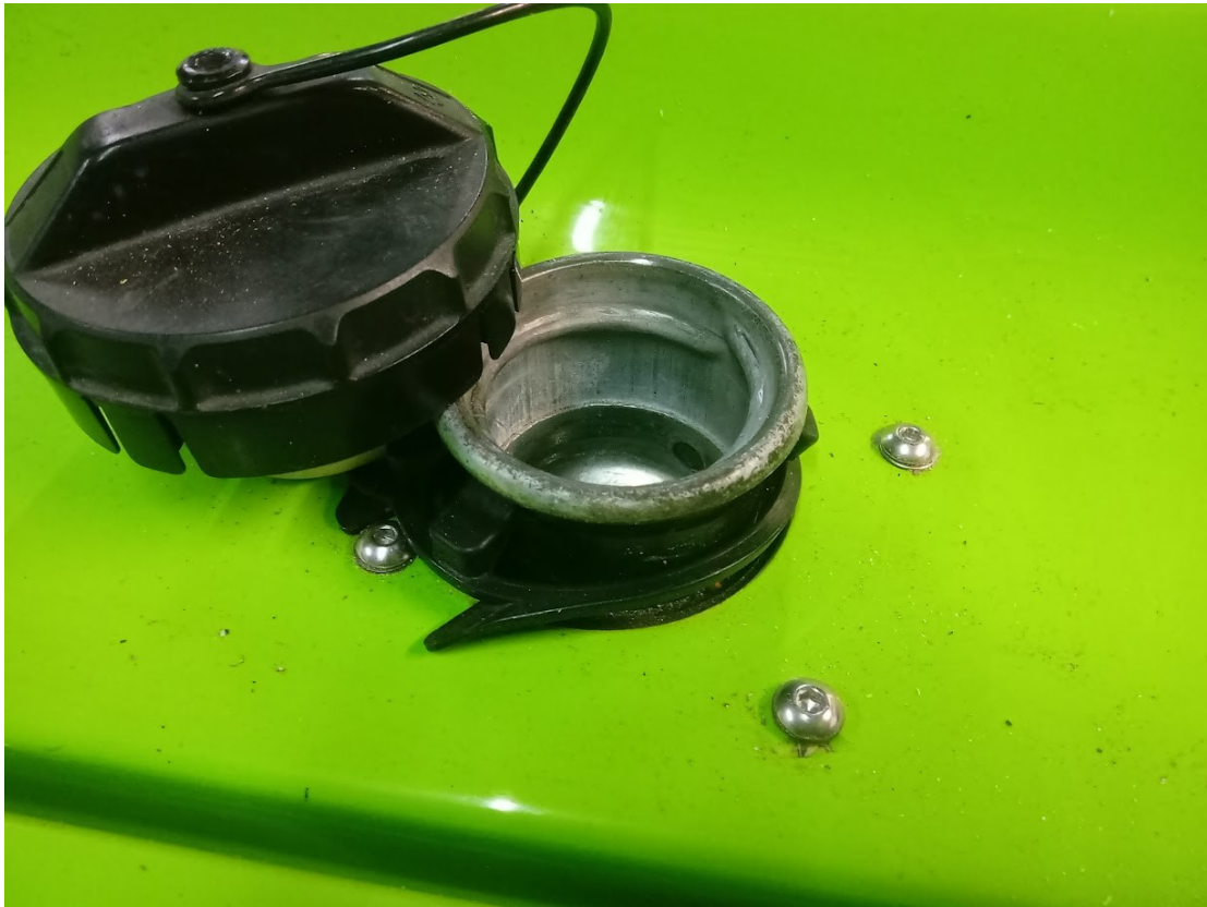
Bolt filler pipe for pre-cut hole in body
