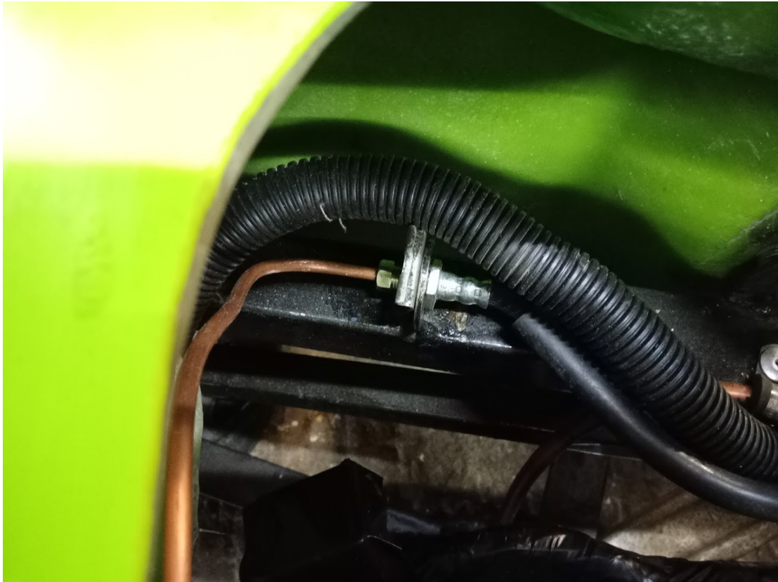
Couple up clutch hydraulic bundy to bracket welded to top of chassis
