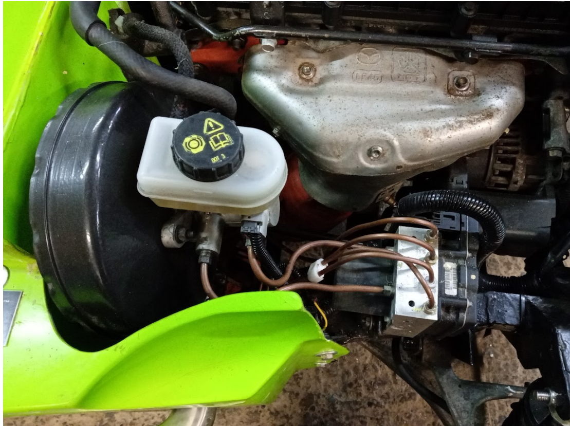
Fit servo thru precut holes in bulkhead, attach pedal box and bolt up
