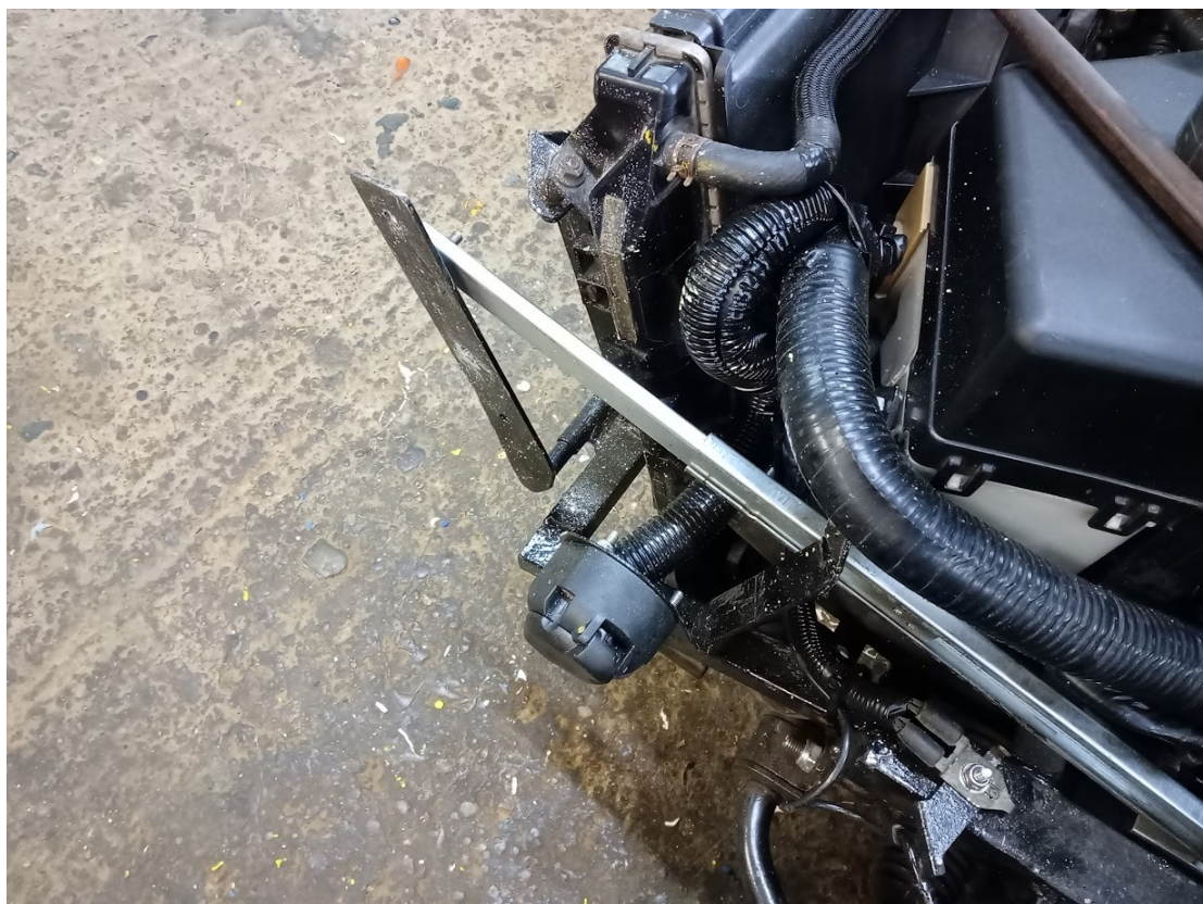
(the steel ratchet bonnet stay is factory fitted)
