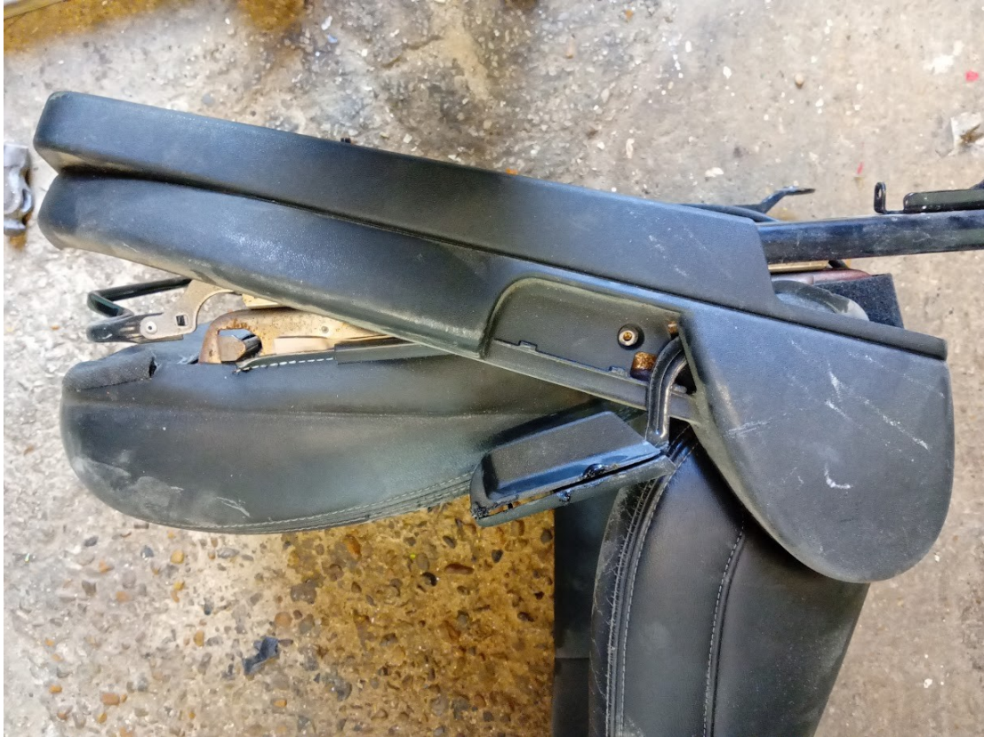
Grind thru lever handle and discard. Discard black plastic side panel
