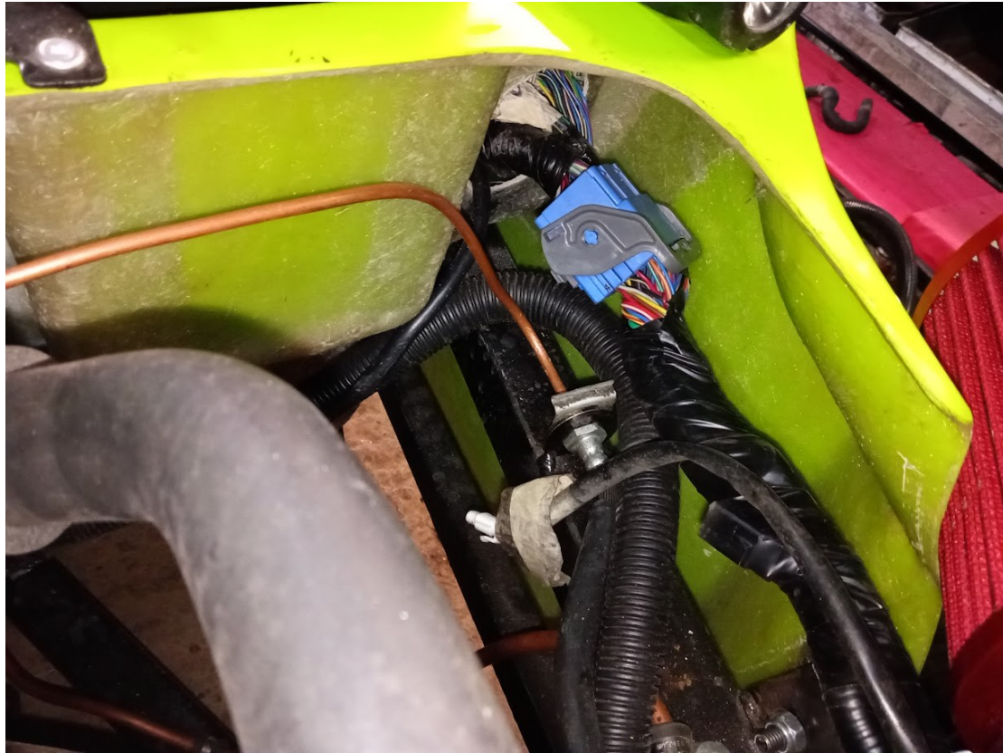
Couple up engine harness left side thru precut hole viewed from engine side
