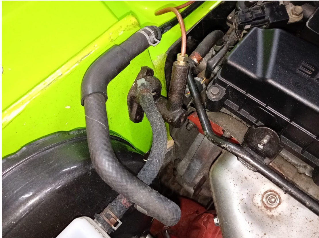
Fit clutch master cylinder thru precut holes in bulkhead, attach pedal box and bolt up, couple up hose to reservoir
