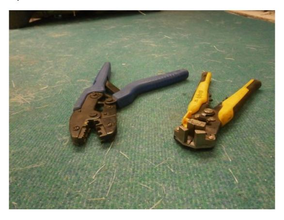
You must use proper wire crimping tool. NOTE 1/2" wide jaws to crimp wire AND outer cover rather than the cheap 1/8" wide jaw type that do not fully crimp. The yellow plastic outer cover stripper is adjustable and saves time.
